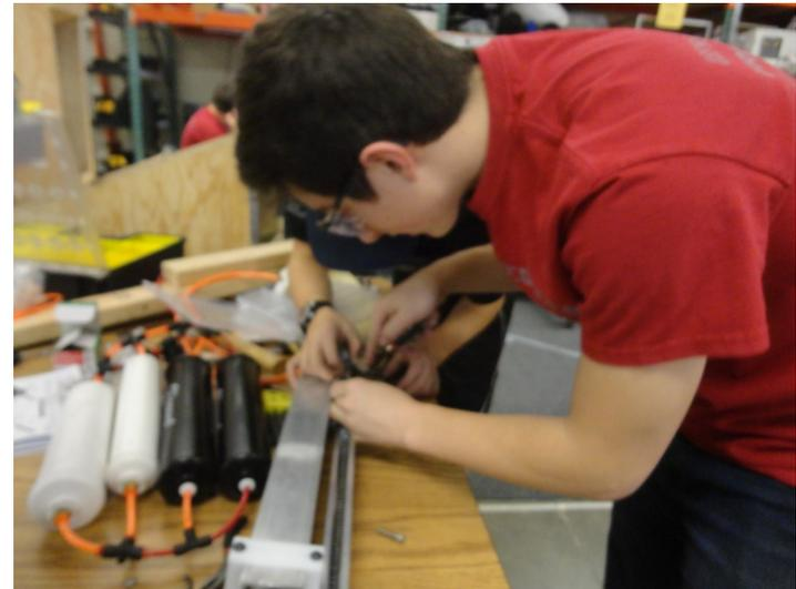
The pushing mechanism is made up of two 1.5 in cylinders with a 15 in stroke. There is a chain mechanism allowing us to achieve a double extension of 30 in.
