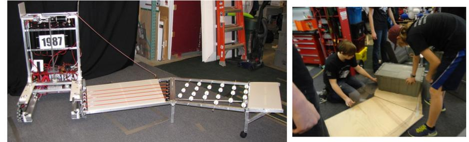
The first part of the conveyor has both passive rollers, as well as a powered carbon fiber roller, and the final section is driven by a Bane Bot motor.
